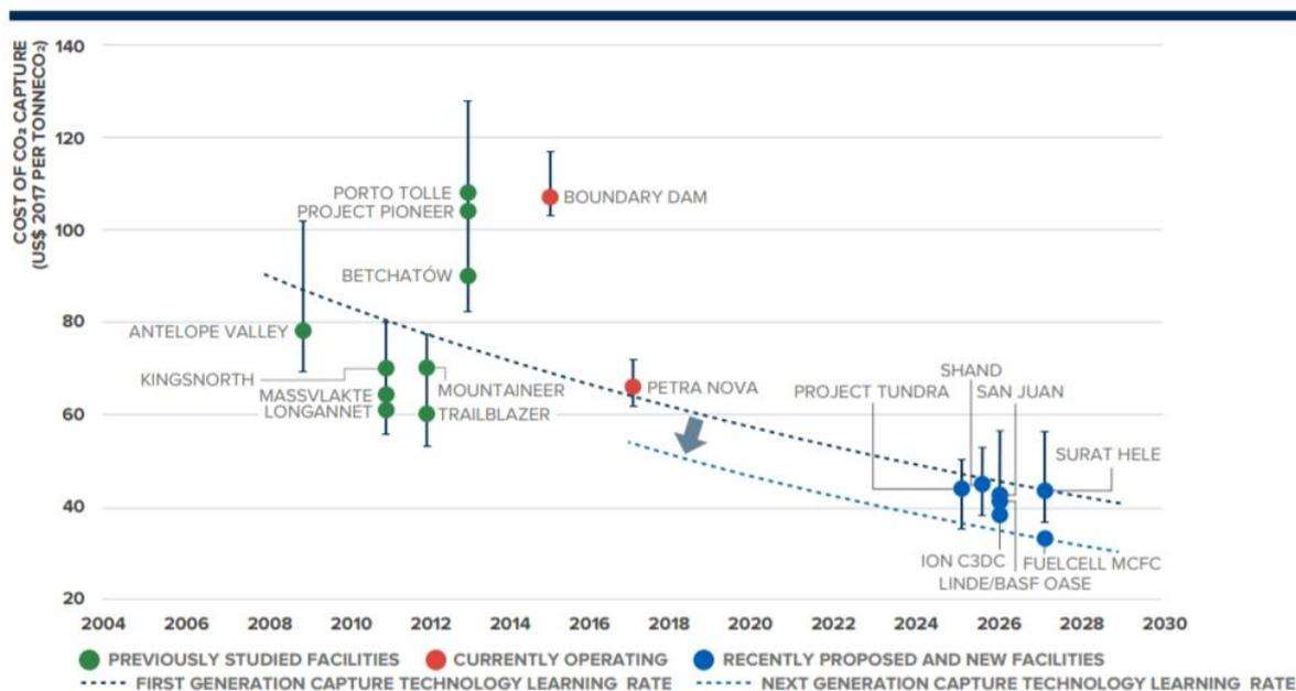
Figure 2: Levelised cost of CO<sub>2</sub> capture for large-scale post-combustion facilities at coal-fired power plants, including previously studied facilities from the Global Status of CCS: 2019.
