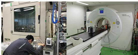
Coreflooding apparatus for relative permeability measurement at JOGMEC Technology Research Center
