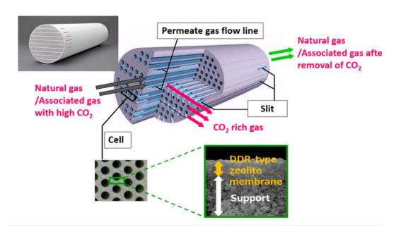
Structure of Large-Size Elements of the DDR-Type Zeolite Membranes Source: 2019 news release | JGC Holdings Corp.
