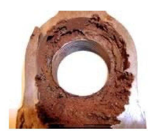
➤ Free water combined with the high CO2 pressure may cause severe internal corrosion in pipeline due to the formation of carbonic acid
